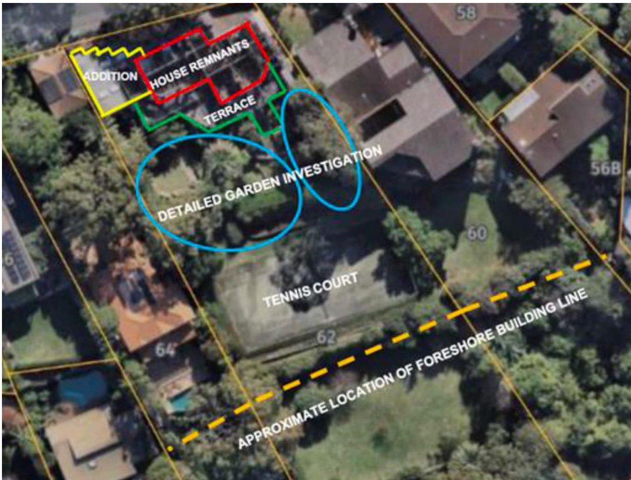
Figure 11 – House and addition (in red and yellow respectively) to be demolished and rear Terrace (in green) to be retained.
